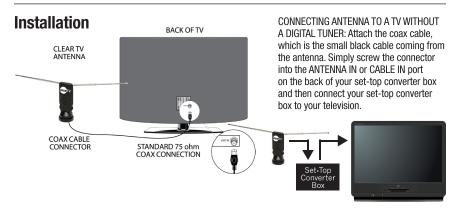
CONNECTING ANTENNA TO A TV WITH A DIGITAL TUNER: Attach the coax cable, which is the small black cable coming from the antenna. Simply screw the connector into the ANTENNA IN or CABLE IN port on the back of your television.
